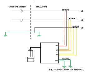
Warning: The AVT must be installed correctly and grounded as described in the installation instructions to provide proper indication of absence of voltage. Sensor leads, including ground, must not be mechanically connected to each other in order for the device to verify connection to the circuit.
